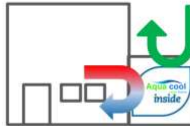
100% Air recirculation with independent scavenger air flow
